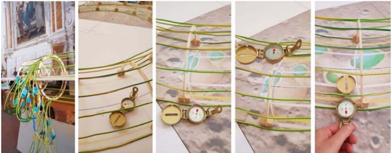
Figure 4. Some views of the scale model realized to demonstrate the absence of magnetic field inside the toroidal arranged cable frame.
